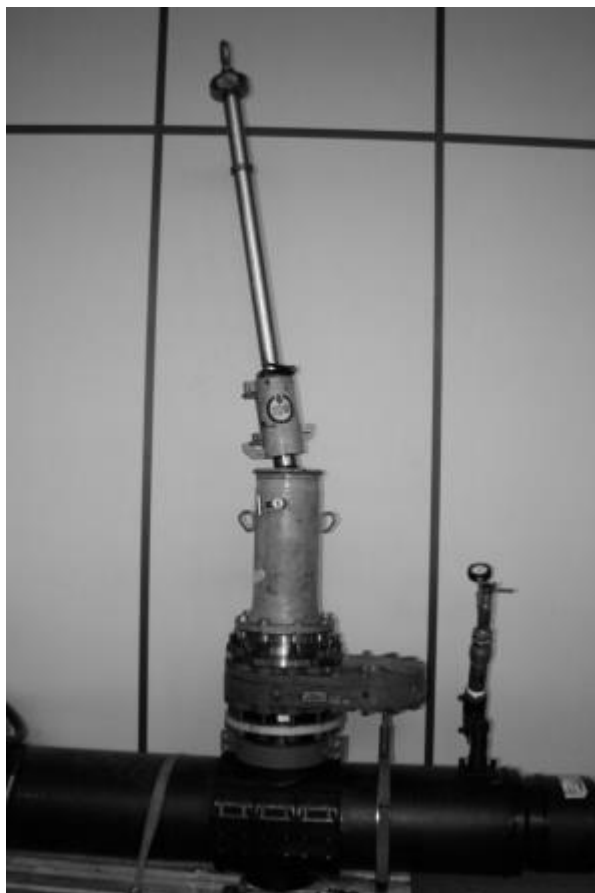
Figure 38. Install Plugging Machine ( valve design will be changed after September 2019 )
