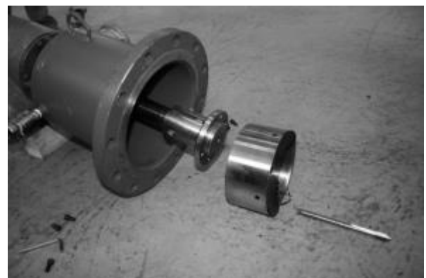
Figure 8. Cutter holder, cutter and pilot drill
